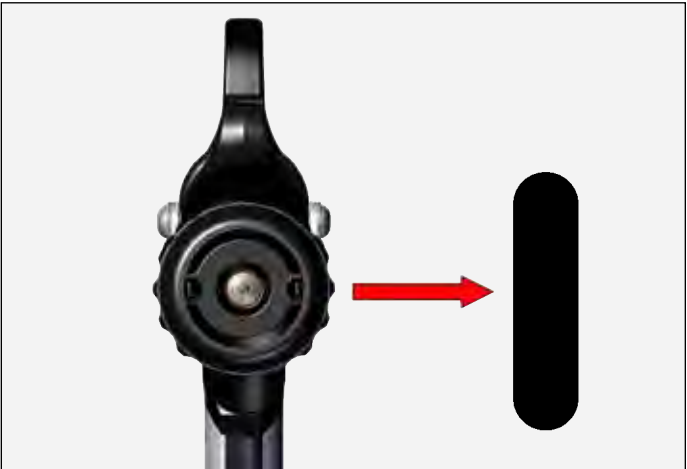
(Horns Aligned Horizontal)
